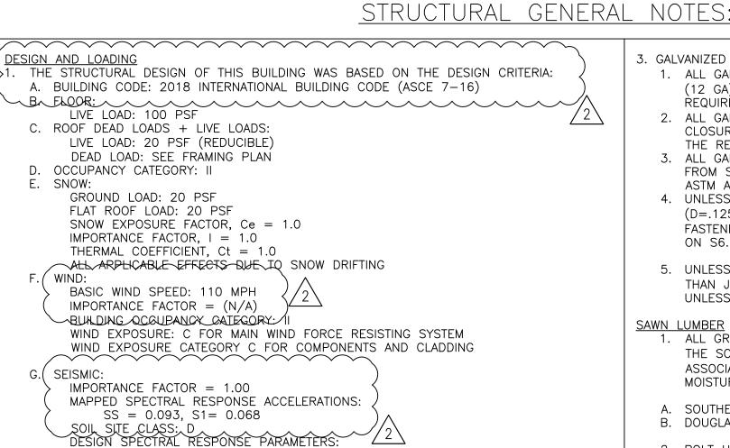
SEISMIC FORCE RESISTING SYSTEM: STEEL ORDINARY MOMENT FRAMES RESPONSE MODIFICATION FACTOR R = 3.5ANALYSIS PROCEDURE USED: EQUIVALENT LATERAL FORCE ANALYSIS
