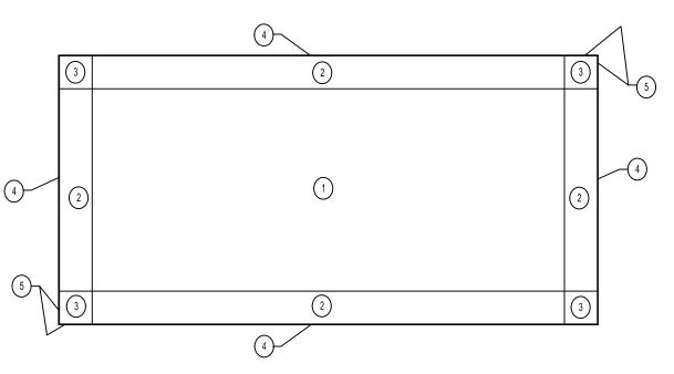
COMPONENTS & CLADDING WIND PRESSURE DIAGRAM
