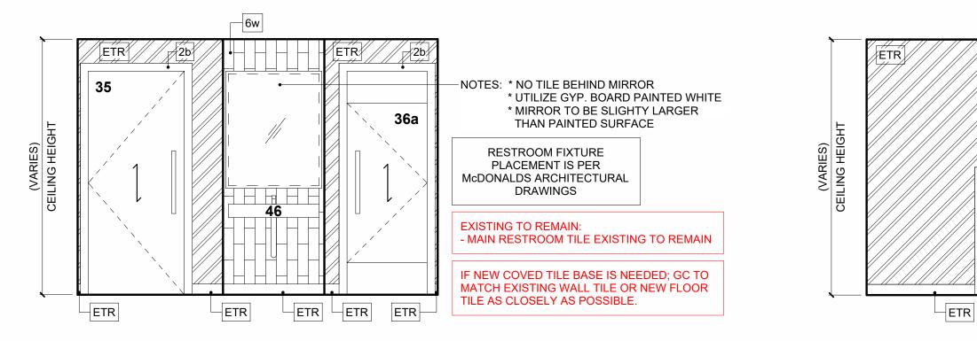
TYPICAL RESTROOM ELEVATION (NOT FOR LAYOUT OR FIXTURE PLACEMENT) FOR REPRESENTATION ONLY
