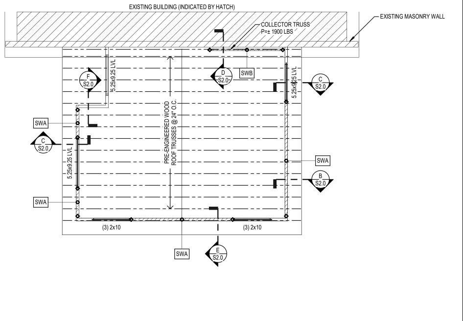
ROOF FRAMING PLAN Scale: 1/8" = 1'-0" A S2.0
